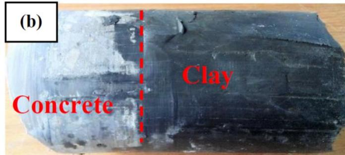
Figure 2. In-situ interface between concrete and clay from the HADES laboratory. The materials have been in contact for 14 years (picture from Phung et al., 2018)
